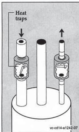
Heat traps, or one-way valves, can control the flow of water into and out of your storage tank.
