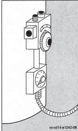
Timers that automatically turn your water heater off and on are a good energy-saving option if you have an electric water heater.
