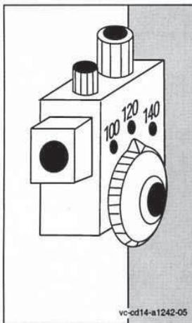
Setting the thermostat on your water heater to 120°F, which is sufficient for most household needs, is an energy-saving measure you may wish to consider.
